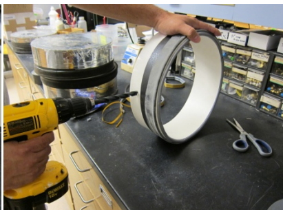
Fig. 14. Hole is drilled in side of chamber top.
