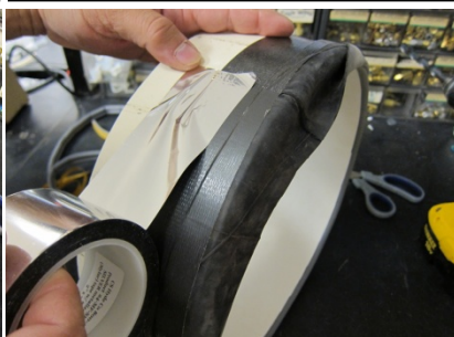
Fig. 20. Reflective mylar tape applied to chamber side.
