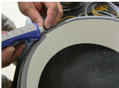
Fig. 13. Edges of weather strip are sealed with glue.
