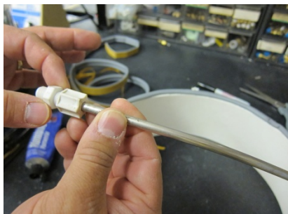
Fig. 16. Plastic union serves as vent tube fitting.
