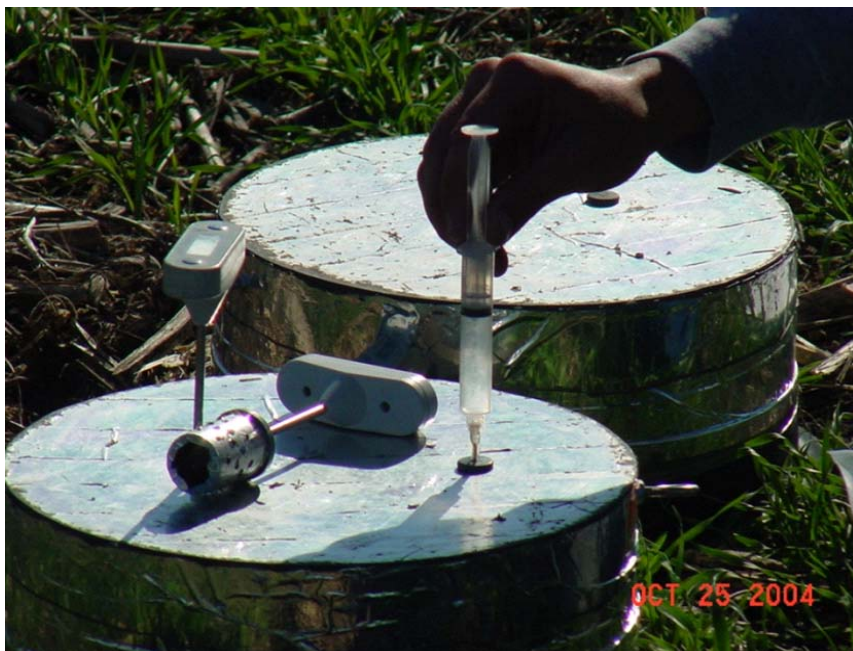
1 Gas sample collection from chambers at Ames, IA location. Thermometers are measuring air and chamber headspace temperatures.
