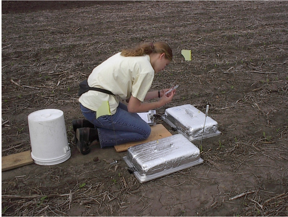
Stainless steel chamber tops (above) and anchors (below) used in St. Paul, MN. Chamber anchors are nearly flush with soil surface. See Appendix IV for construction details. Photos on following page shows inside of chamber top and sample collection method.
