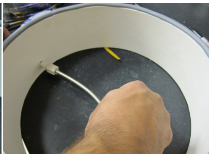
Fig. 18. Stainless steel (1/4") is attached to plastic union.
