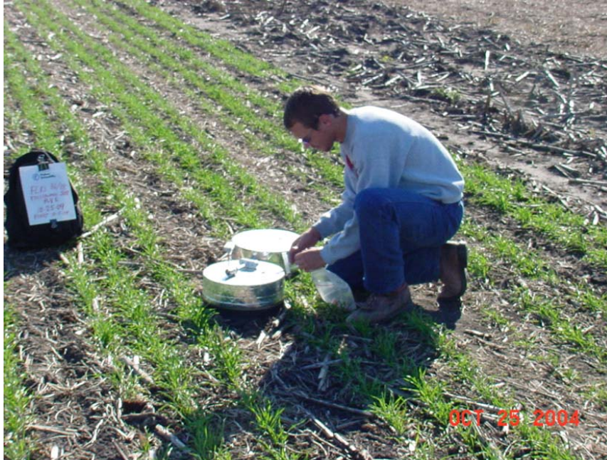
1 Gas sample collection from chambers at Ames, IA location. Thermometers are measuring air and chamber headspace temperatures.
